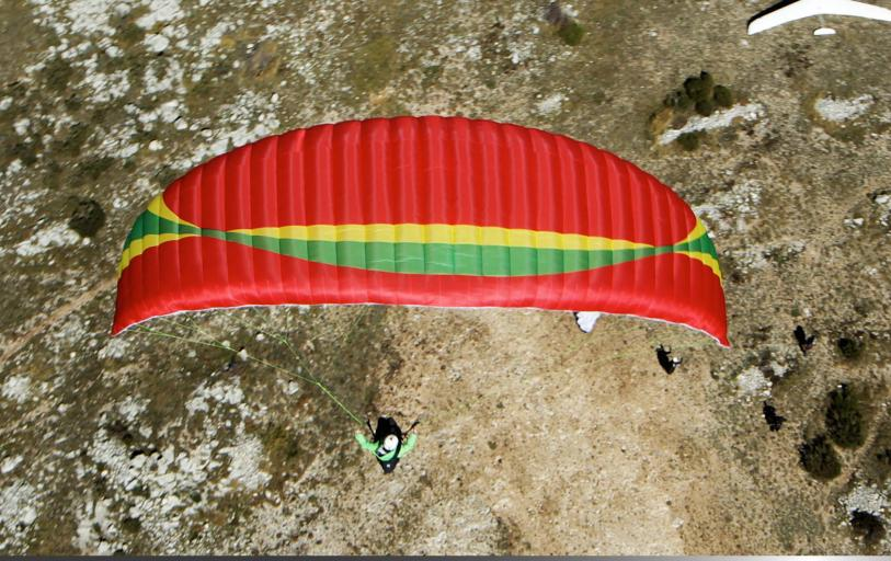
The Adam A, a beginner's wing using 3D Shaping technology and mini ribs.
