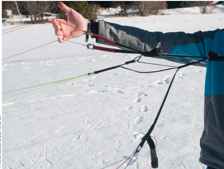
A basic riser: A, A', B and C.
