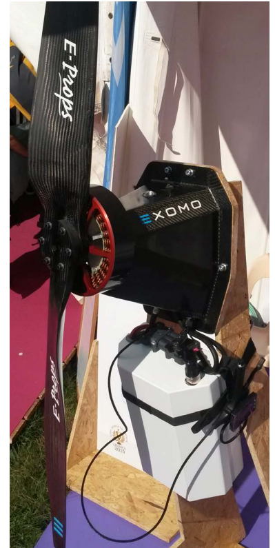
Above, the integral model. An Exomo basic pack of 15 kW, as on the right, with a 45 Ah battery, costs 11430 €.
