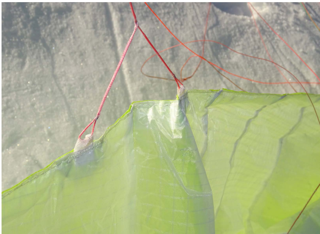
The trailing edge has been sewn without a strip.
