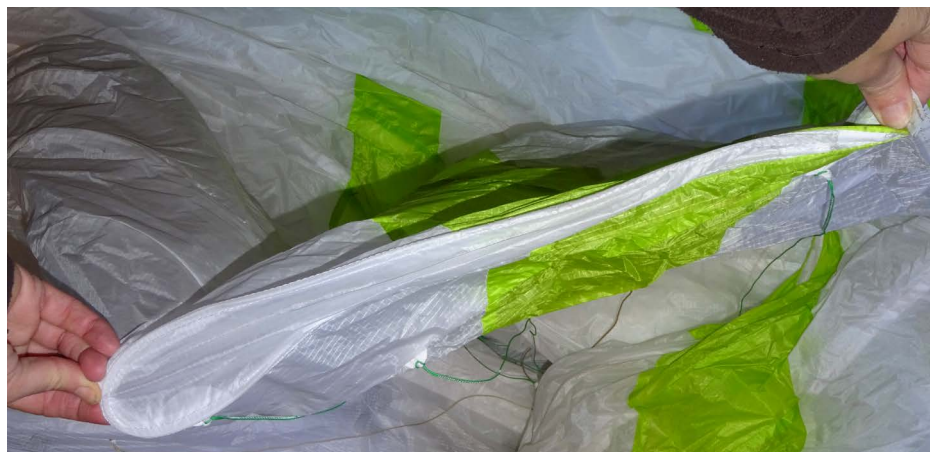
This strange rod in the stabilo, giving a full profile, has a fairly aesthetic function according to the manufacturer. Photo: S. Burkhardt
