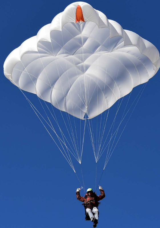
A steerable square reserve, the "Diamond Cross" by Charly, coming in to land at the Stubai Cup.
