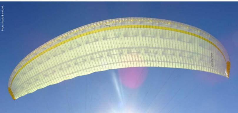
To accommodate 99 cells into a wing with a low aspect ratio, the cells need to be very narrow.
