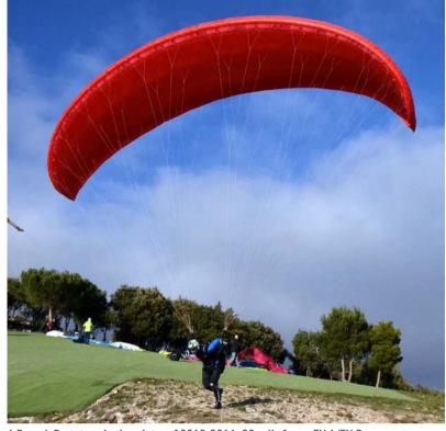
A Papesh Prototype in the winter of 2015-2016: 90 cells for an EN A/EN B.
