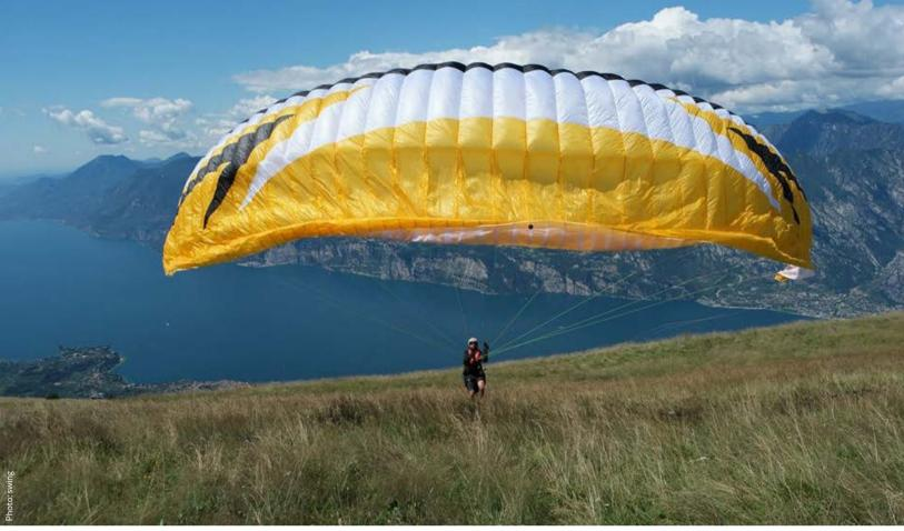
Clearly visible: the back fills later, the RAST rib fulfils one of its roles.
