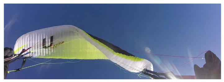
The wing is very well behaved during small collapses, taking a bit more bank after a bigger collapse, photo taken from a video: Estéban Bourroufiès.
