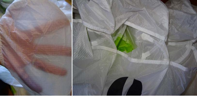
The fabric is a mix of Skytex 38 g/m2 and Dominico D20 35/m2, and the manufacture is more tough than lightweight. Photo : S. Burkhardt
