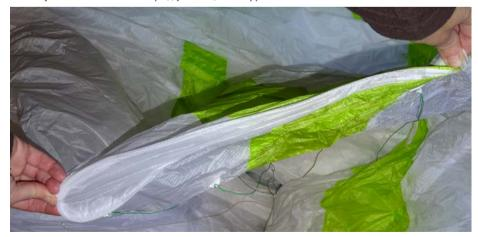
This strange rod in the stabilo, giving a full profile, has a fairly aesthetic function according to the manufacturer. Photo: S. Burkhardt
