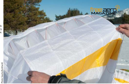
Despite being made principally from light weight material, it has, all the same, Mylar film.
