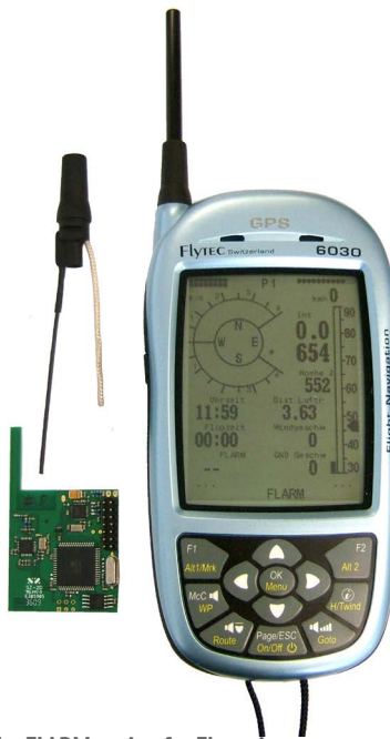
The FLARM option for Flytec instruments. www.volirium.com
