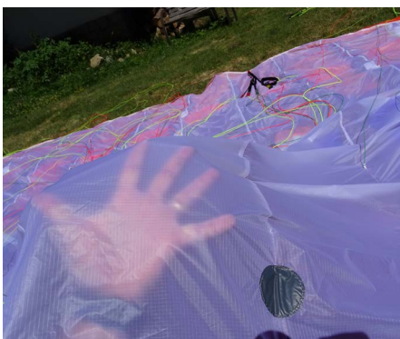
The fabric used for the lower and upper surface, despite its transparency, is Dominico 30D. It's obviously strong.
