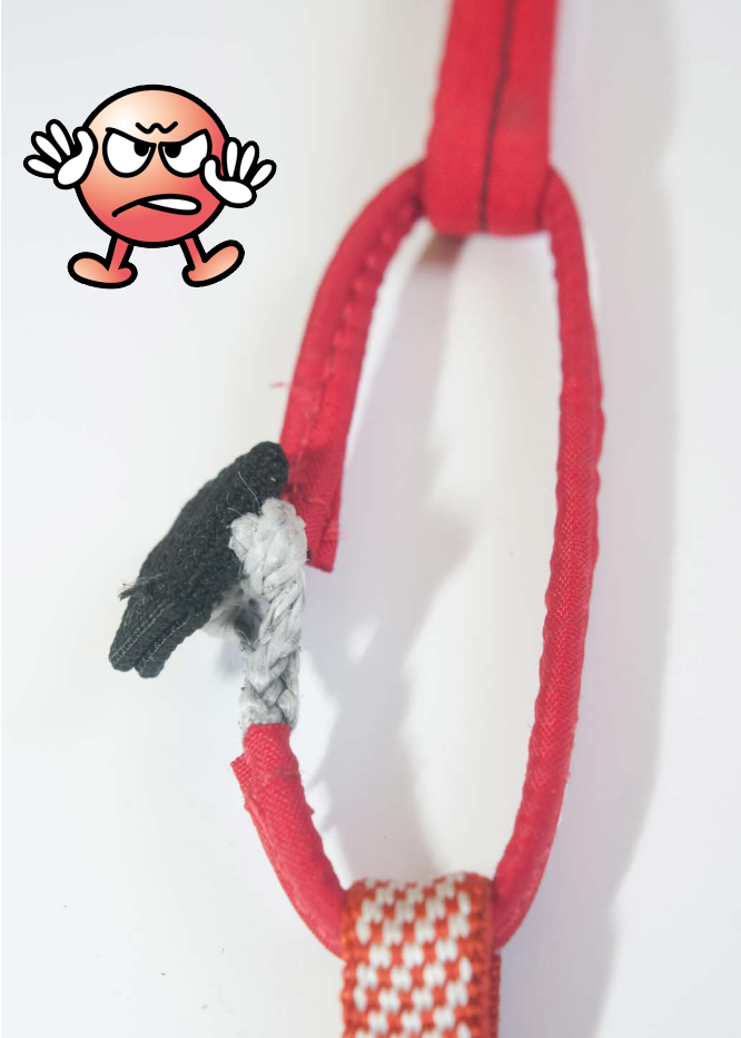
Not good: The softlink has been fastened correctly, but the strap has only been looped round once. Its resistance has therefore been halved: 1150 kg instead of 2300 kg. (Admittedly, it's still better than a poor quality maillon...)
