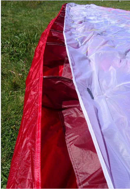
A leading edge with openings which suck up the air by themselves and made from very strong materials: a solid wing.
