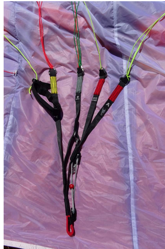
Relatively few lines, risers which are very simple to understand and, in addition, clearly marked (A,B,C...)
