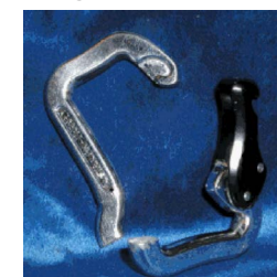
The problems fifteen years ago started on the Parafly chromes (left). The karabiners broke during take off.
