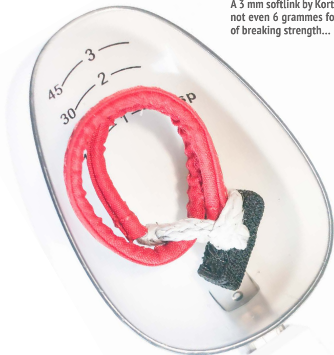
A Dyneema/Dyneema/Dyneema connection: very strong and reliable if the softlink is of good quality.
