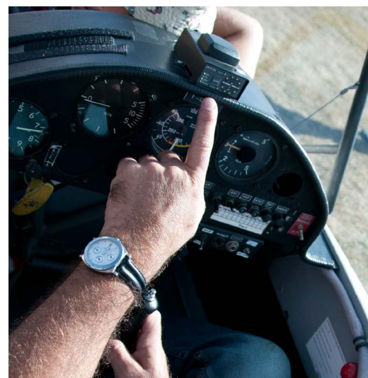
FLARM in a sailplane. Photo : S. Burkhardt
