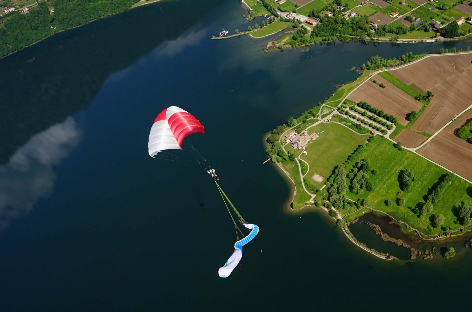
A Rogallo: a lower sink rate, more horizontal trajectory and steerable, but a bit more complex than a simple round or square parachute.
