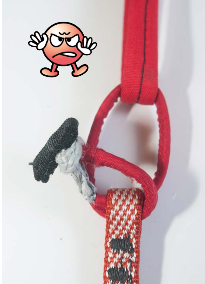
Not good: It is fastened correctly, but the softlink hasn't been correctly looped round twice. The same result as on the left: The resistance is halved.
