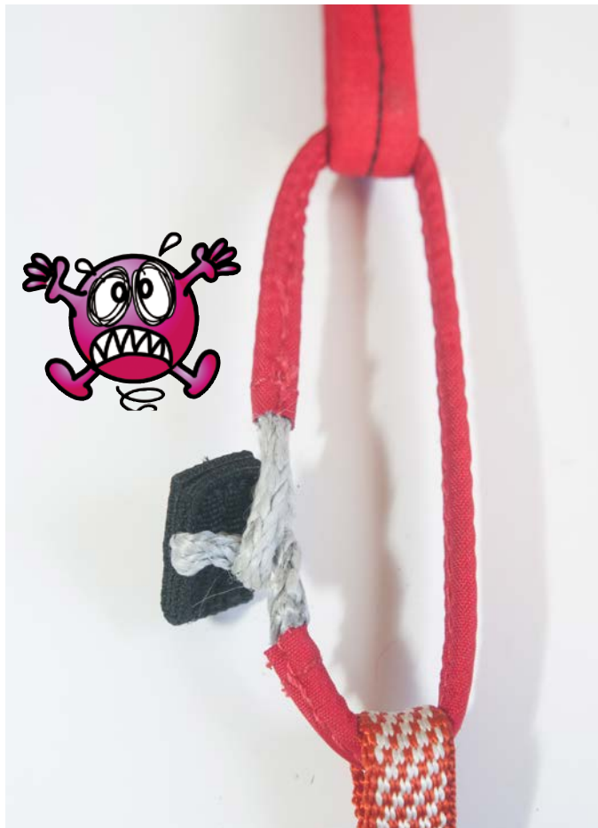
This is really bad: The softlink has only been looped round once, it has been incorrectly fastened, and the tab is about to come out of the other loop...Not good, not good at all...
