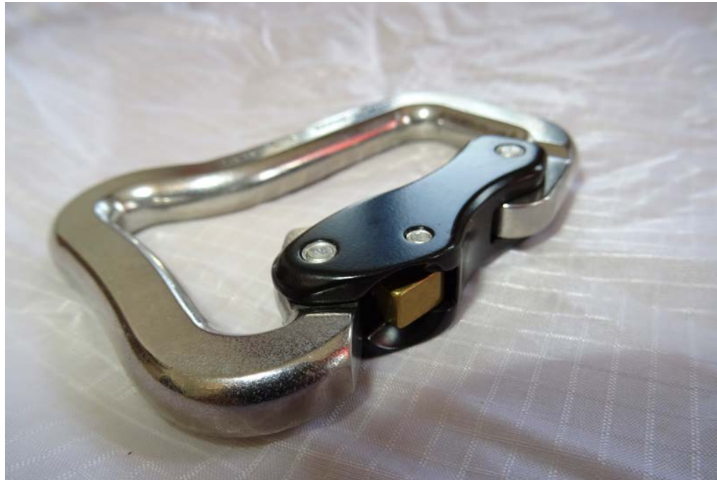
A stainless steel Para-fly: these karabiners were a good answer to the problems encountered at the time. Disadvantage: the weight is nearly three times higher than an aluminium karabiner (about 140 g). They are also very well suited to paramotor trikes.
