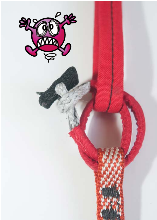
Very bad: The softlink has been correctly looped round twice, but not correctly fastened: The loop without the tab has just been put OVER the loop with the tab. It hasn't gone THROUGH the loop with the tab first. It may hold once under tension, but coming undone unexpectedly can't be completely ruled out.
