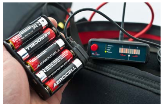
One of the first portable FLARMs, tested by free.aero . You had to take a 12 V block of batteries.
