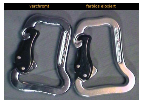
The problems fifteen years ago started on the Parafly chromes (left). The karabiners broke during take off.
