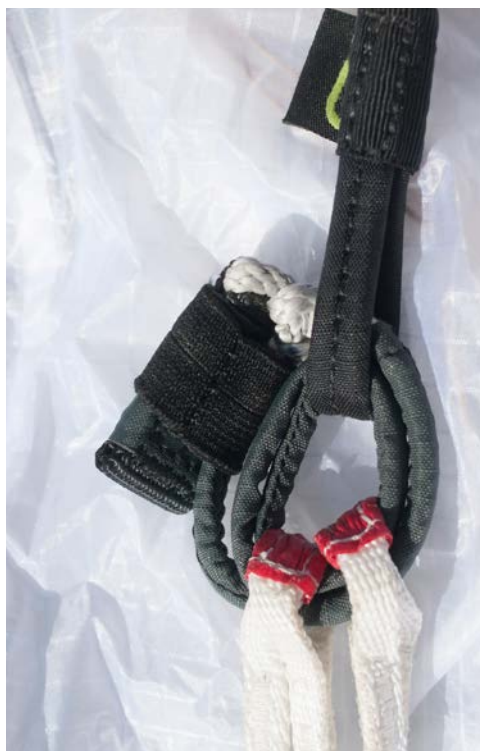
A Dyneema/Dyneema/Dyneema connection: very strong and reliable if the softlink is of good quality.
