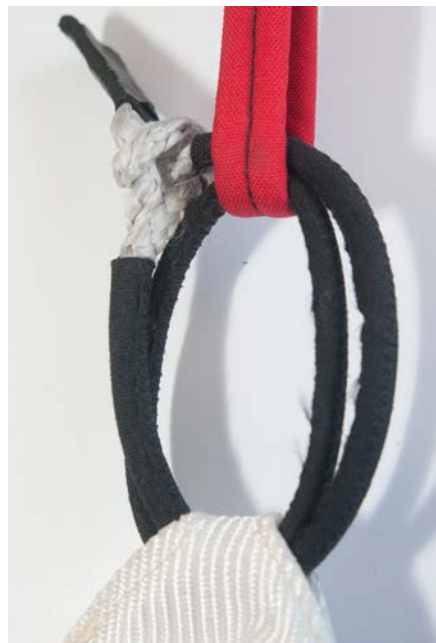
One of the first flexible connectors for paragliding: Bertrand Maddalena, then owner of Ripair, designed it twelve years ago. Most paraglider pilots were fairly sceptical. However, this connector only weighs 12 grammes, and has a breaking resistance of 2.2 t. It is more resistant than a typical aluminium karabiner (about 1.6-1.8 t for 70 grammes) and just as resistant as a stainless steel karabiner (130 grammes, 2.2 t).
