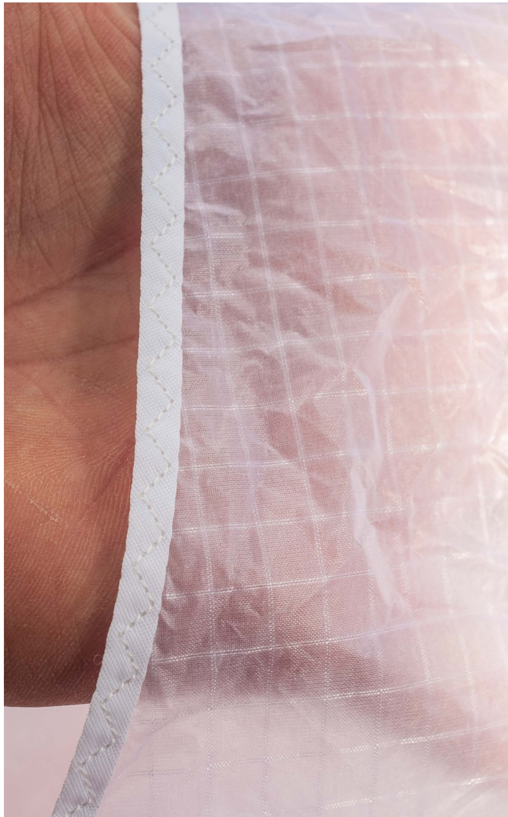
Porcher Skytex 27 g/m 2 on an Advance Pi 2. Photo: S. Burkhardt
