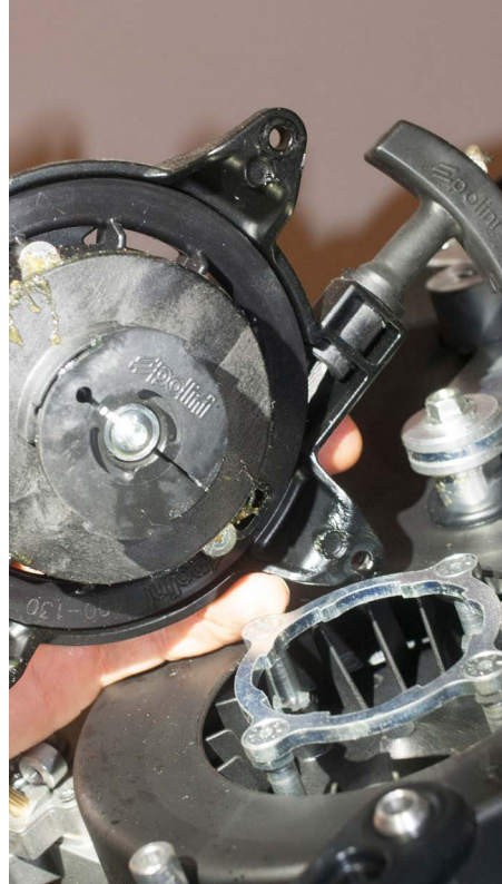
To change the radiator attachment due to an upgrade advised by the manufacturer, we had to take off the Flash-Starter...
