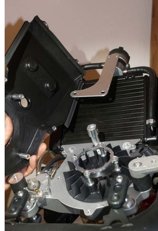
...as well as the cover for the fan (right). Below, the old bushing, further below, the improved attachment which lasts longer.
