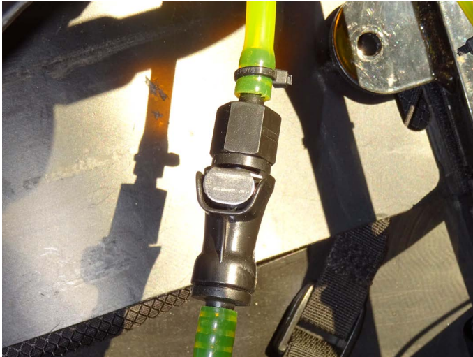
Recommended accessory: a quick connector (about 19€) between the tank and the motor. Also available from Reuter.
