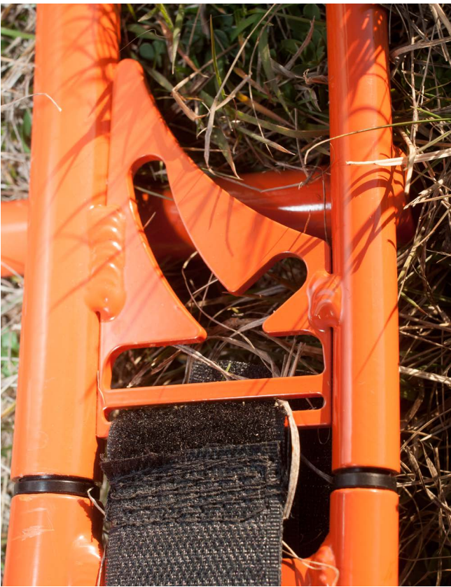
Different diameter tubes save weight.
