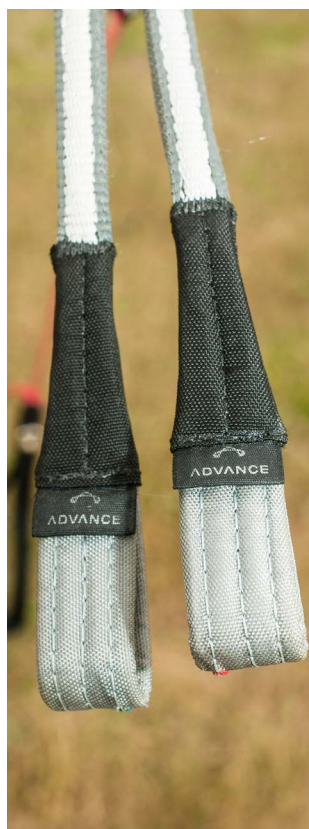
The light risers save 150 g thanks to Softlinks and straps which are a lot thinner. Photos : S. Burkhardt
