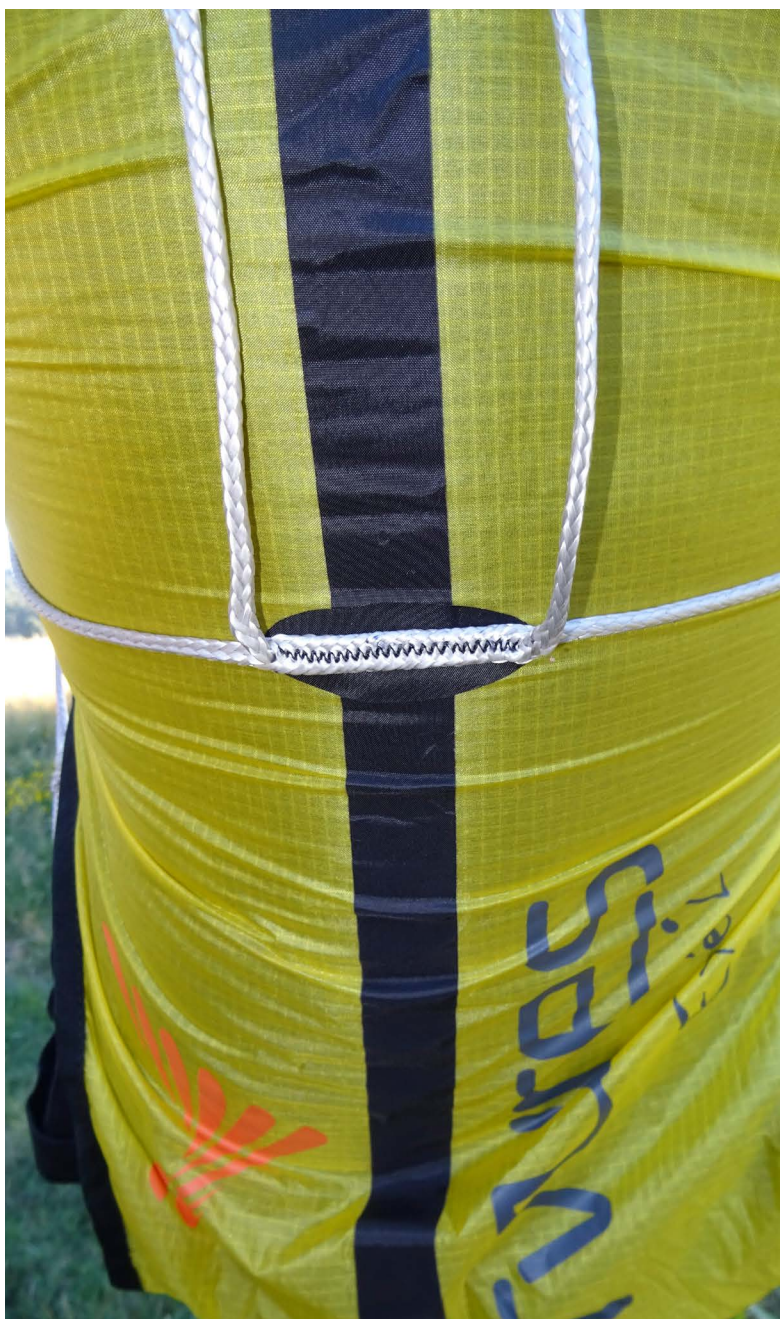
Skytex fabric and Dyneema: the typical formula for an impressive reduction in weight.
