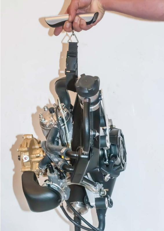
In the office, the Polini Thor 80 weighed 11.6 kg. It isn't ultra light, but very good for a motor this powerful! The radiator is integrated with the motor, making it very compact.
