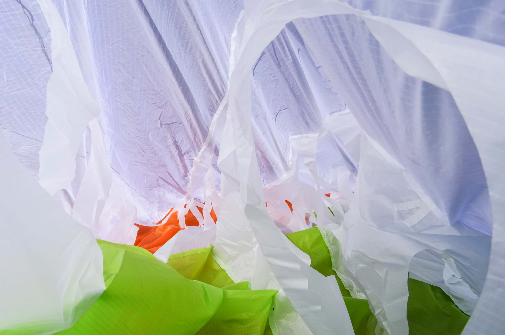
One of the ways of reducing weight: open up the cell walls.
