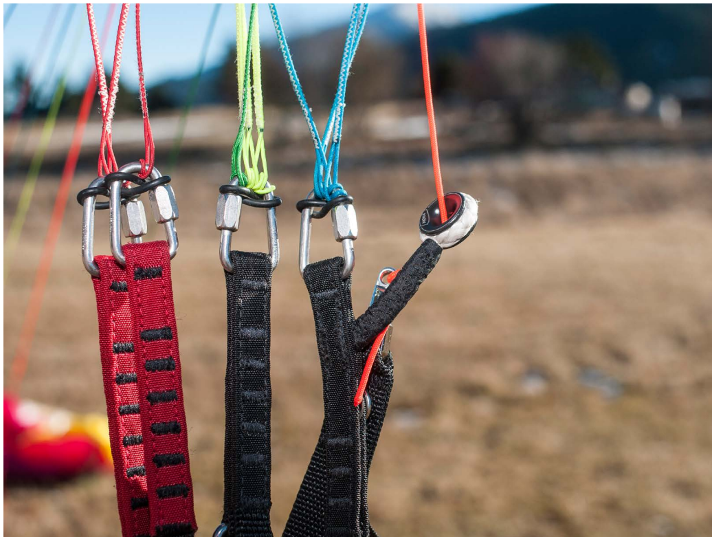
Classic maillons and risers, with classic but narrower straps. The advantage compared to the Dyneema risers which are lighter still: the classic ones are easier to use. Photos : Burkhardt
