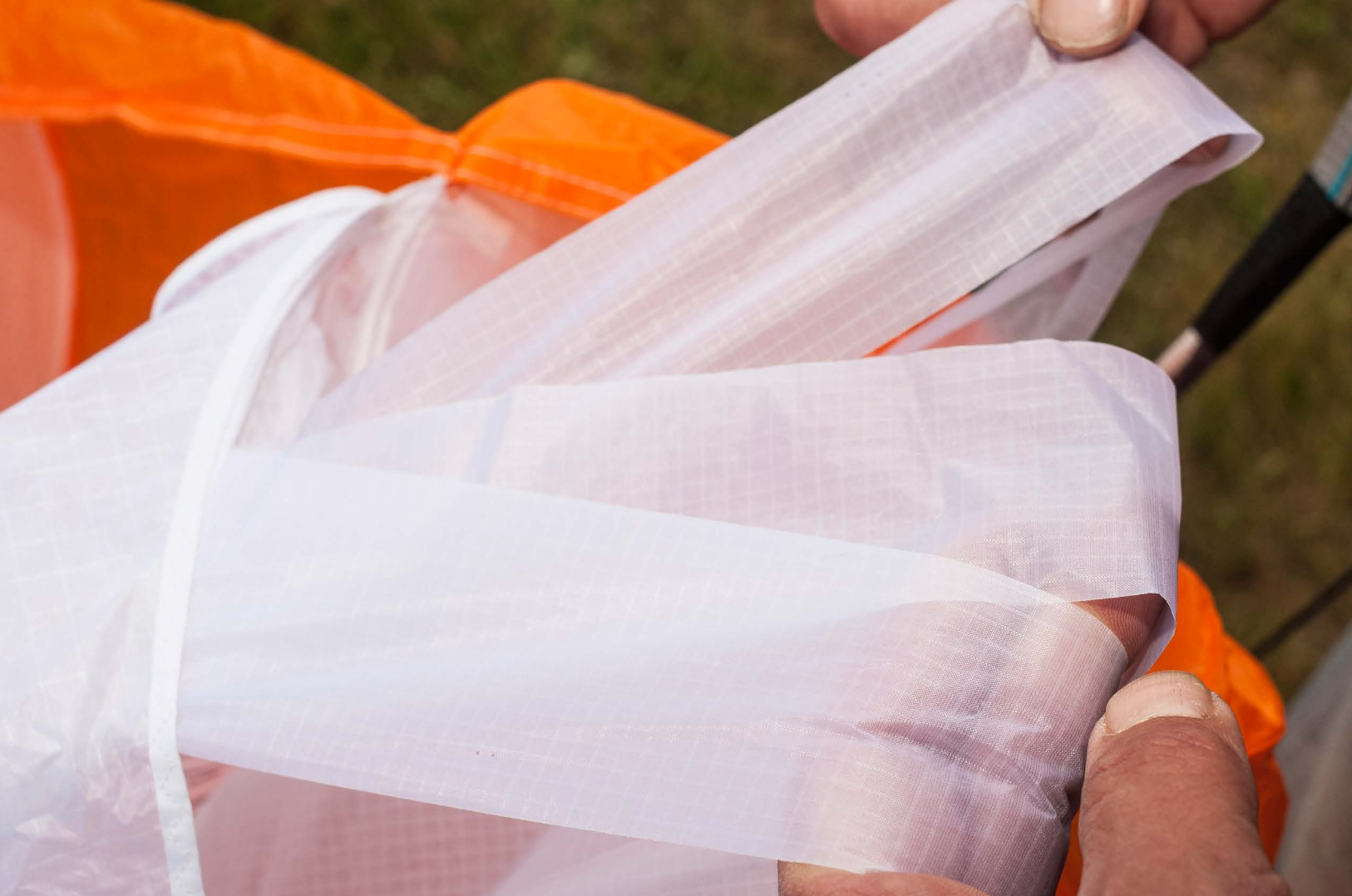
The famous Sliced Diagonals. Instead of just one piece of fabric for the diagonals, these ones are made up of thin bands orientated in the direction of the force. This makes the wing lighter and can give the profile a longer life expectancy. Photos: S. Burkhardt
