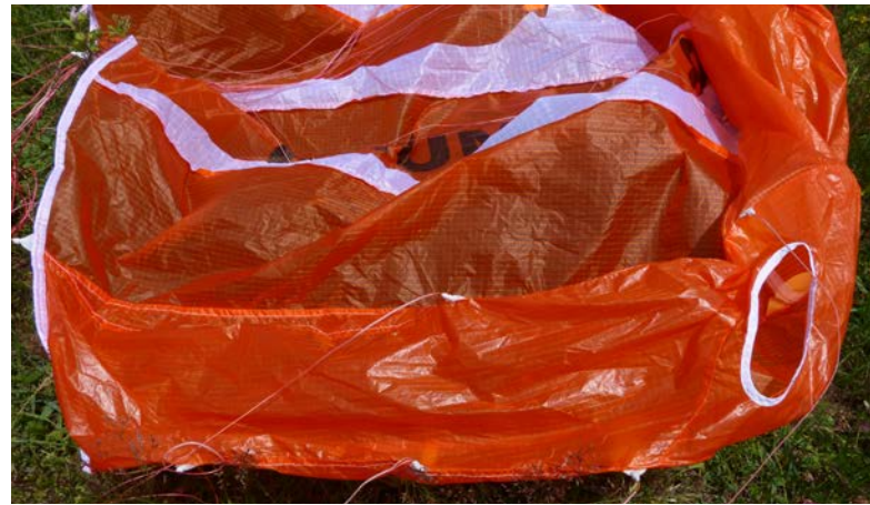
One cell plus two mini cells, pyramidal lines, everything is light on this Skyman 20: only 1.59 kg But the materials have been chosen accordingly: the Dominico 10D fabric seems particularly thin (but very silky).
