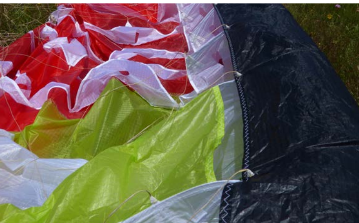
Six cells, four rows of lines, metal (Nitinol) leading edge rods and some Skytex 27 on this "Plume" version of the Skin 2. The 18 weighs 2.13 kg on our scales. It's a featherweight, but 500 g more than the Skyman. An even heavier version exists: 2.5 kg made with Skytex 32 fabric.
