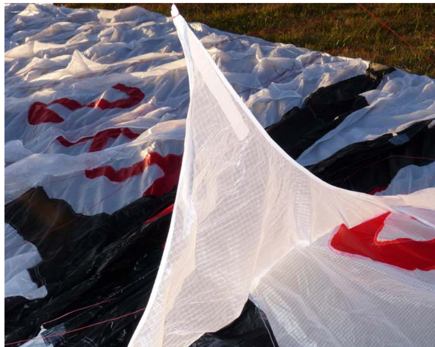
Contrary to their solo wings, for the Sir Edmund tandem, Skyman added trim on the edges of the cells.
