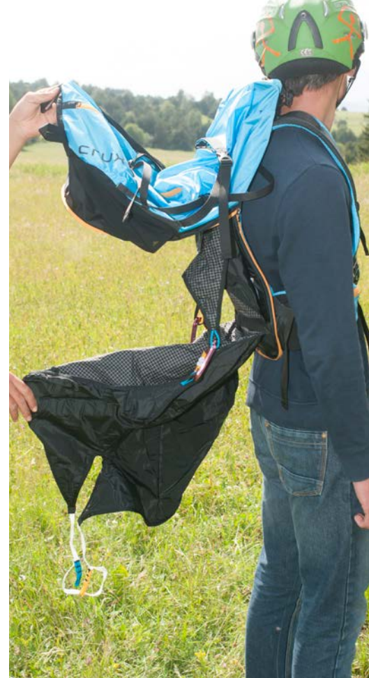
Transforming the bag into a harness: open the lower compartment, the leg straps fall out, the pilot puts the harness on...
