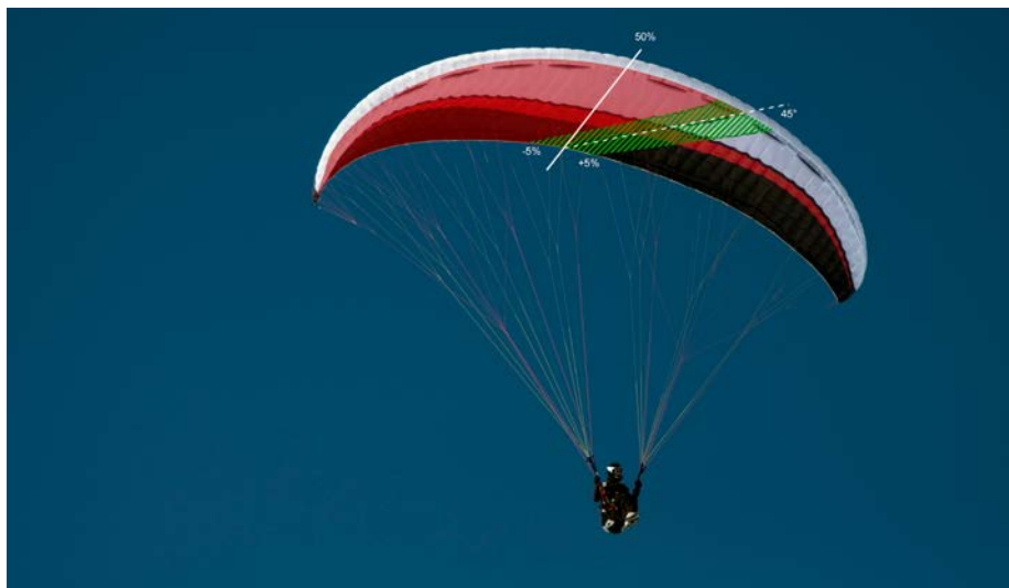
The definition of asymmetric collapses required has slightly changed. Above, everything in red must disappear in the 'big' EN 2005 collapse, with a tolerance (in green). Below, comparing the old and the new collapses. The principle remains the same in the 'new' EN. On the other hand, it forbids folding lines as a way of achieving this, except for EN Ds. Photo: Gudrun Öchsl/Profly
