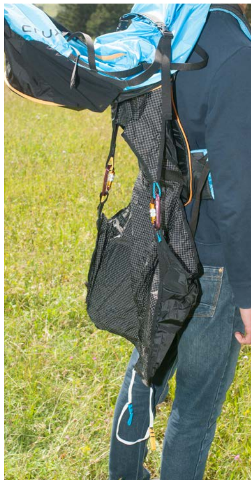
Transforming the bag into a harness: open the lower compartment, the leg straps fall out, the pilot puts the harness on...
