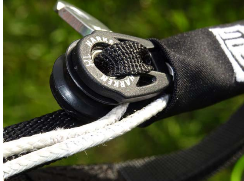
A Harken pulley held in place by a sheath. Impressive detail!
