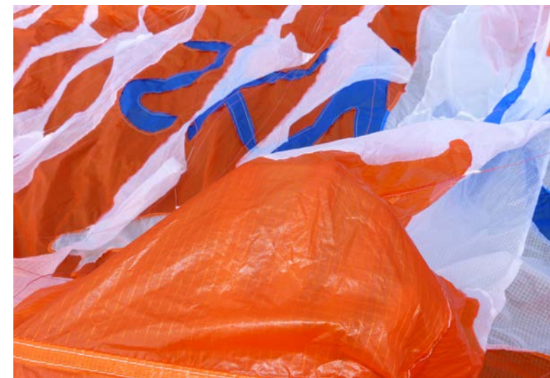
One cell plus two mini cells, pyramidal lines, everything is light on this Skyman 20: only 1.59 kg But the materials have been chosen accordingly: the Dominico 10D fabric seems particularly thin (but very silky).
