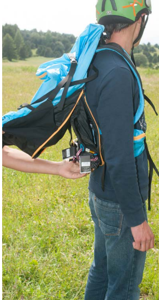
Transforming the bag into a harness: open the lower compartment, the leg straps fall out, the pilot puts the harness on...
