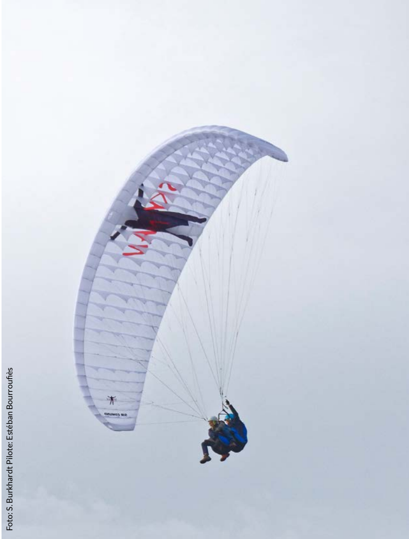
Sir Edmund Bi (2017): A single central cell and a little cell in each stabilo.
