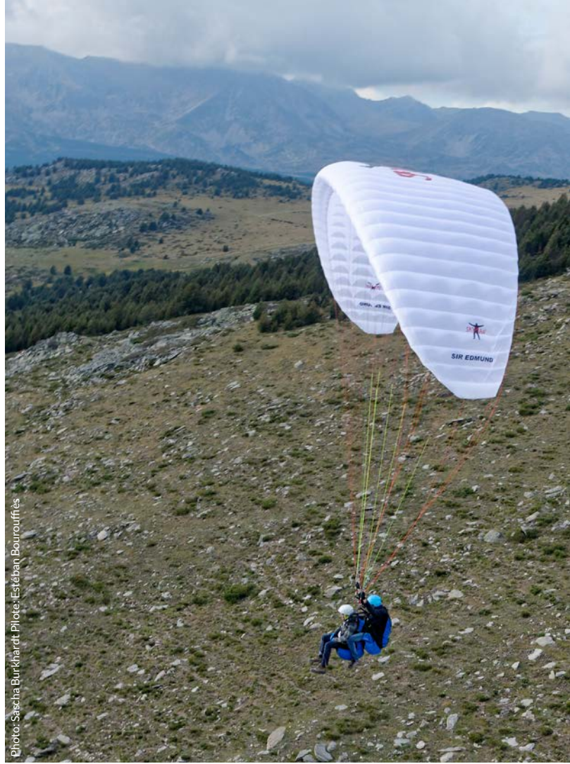
The Sir Edmund Bi (2017): a single central cell and a little cell in each stabilo. The leading edge rods are plastic.
