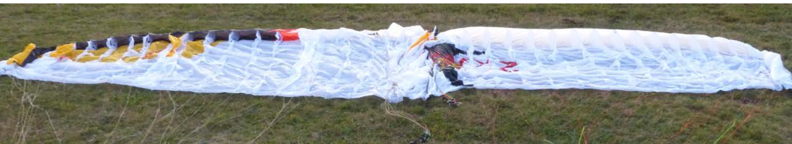
Half a wing of each glider side by side: the Bi Niviuk (left) has got a higher aspect ratio, while the Skyman is more compact. The surface is almost equal.
