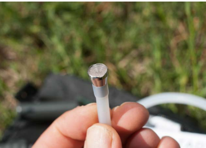
The little inlet tube with the pre-filter.
