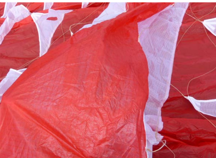
Six cells, four rows of lines, metal (Nitinol) leading edge rods and some Skytex 27 on this "Plume" version of the Skin 2. The 18 weighs 2.13 kg on our scales. It's a featherweight, but 500 g more than the Skyman. An even heavier version exists: 2.5 kg made with Skytex 32 fabric.
