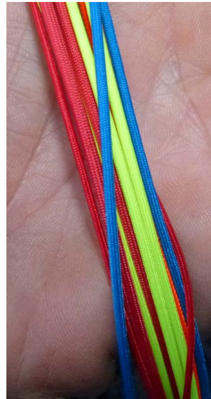
The sheathed lines on the Bi Skyman Pro version.
