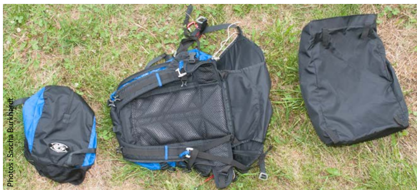
A modular system: the airbag and the compartment for the helmet can be removed.
