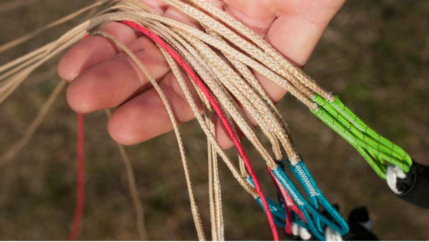
The unsheathed lines on the Niviuk Bi Skin; this material has been tried and tested.
