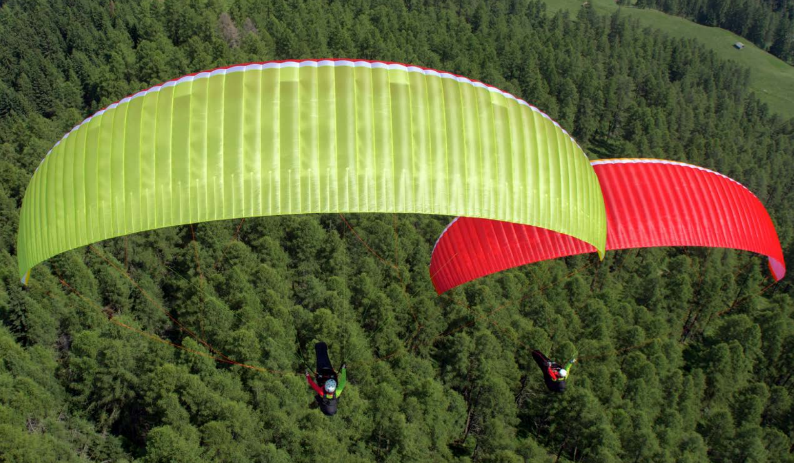
Clearly visible: the mini ribs on the trailing edge as well as on the very airy diagonal cell walls.
