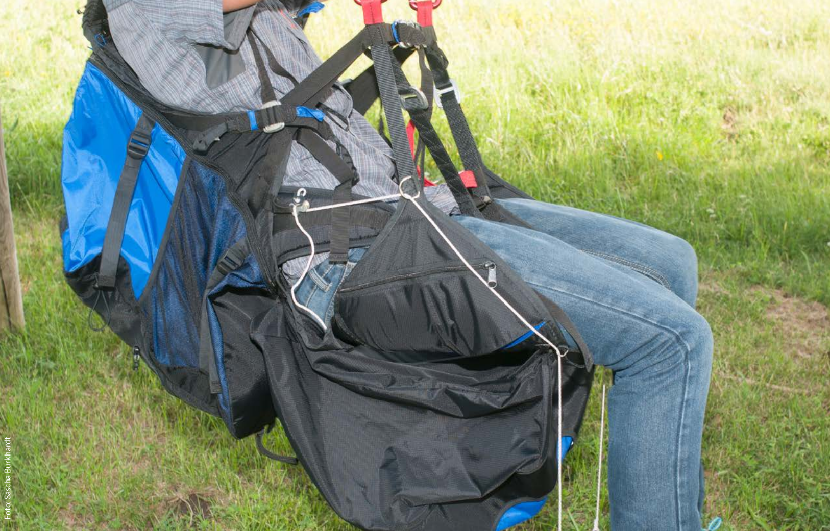
A modular system: the airbag and the compartment for the helmet can be removed.
