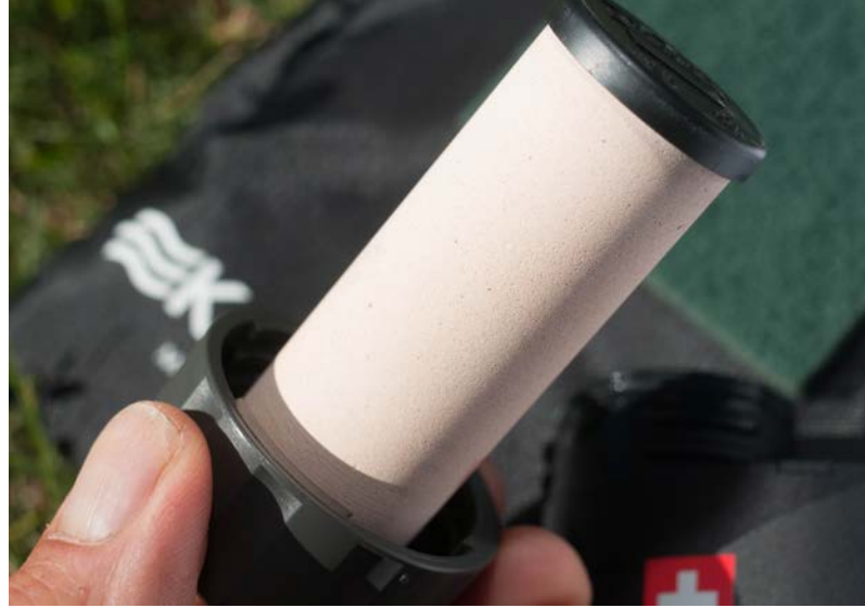
The ceramic filter with 0.2 micron pores (=0.0002 mm). It can be cleaned with an abrasive sponge. Thus it is good for up to 7000 l, then you can throw everything away. But 7000 l is a lot: you would need to pump for ten days, night and day, without stopping.
