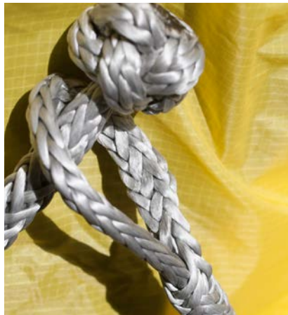
A simpler fastening thanks to a loop and a ball shaped knot.
