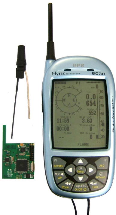
The FLARM module on the old 6030 isn't compatible with the Connect; the latter uses a different one.
