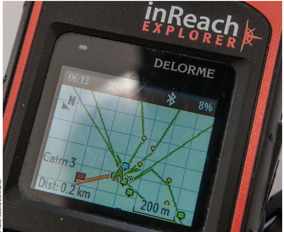
The inReach Explorer offers all the functions on the inReach SE with, in addition, a 'Goto' navigational aid with a graphic display of the track log and messages on the screen.
