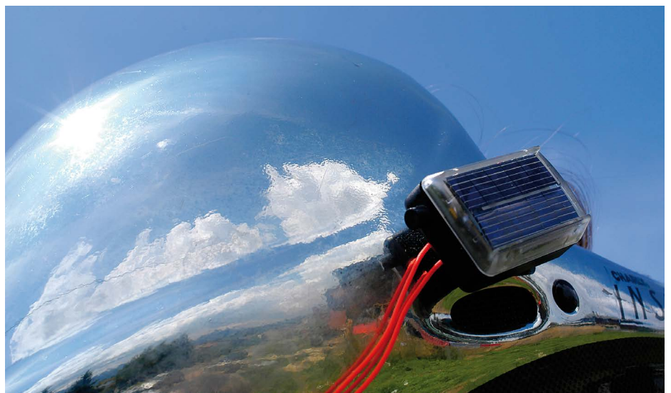
In free flight, to core efficiently, an acoustic vario is the bare minimum. Here's a pioneer in the domain: it came out more than 20 years ago. Even back then, it was just powered by solar energy, well before that was fashionable. It is still on sale for about 140 €. Photo: Sascha Burkhardt
