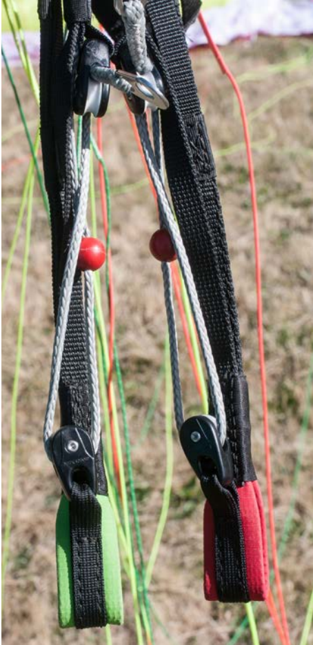
Even on this type of wing, the left/right risers are clearly marked. Also, as is the current fashion, the risers are shorter above the loop.
