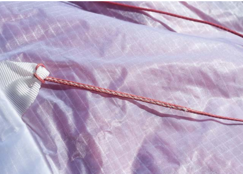
Above, unsheathed lines.
