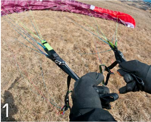
1 The lines are untangled, the risers are parallel and not twisted.
