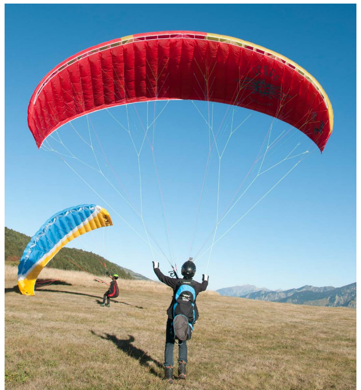
The Kiwi in 2016 (prototype: Furia), is a real little paraglider, but only for on the ground and hops. The wing can be controlled easily with the rear risers ...
