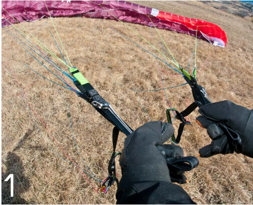
The lines are untangled, the risers are parallel and not twisted.
