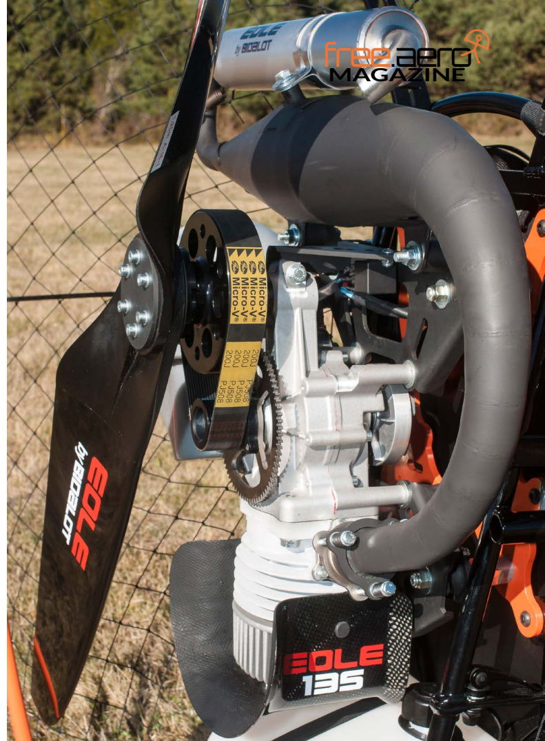
The exhaust pipe: it took more than 15 prototypes to get the result they wanted.
