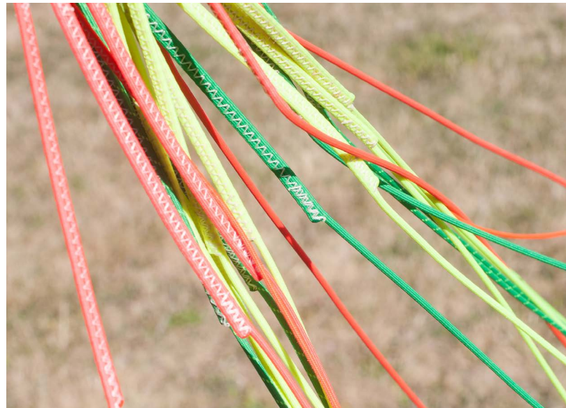
The sheathed lines in the lower part.
