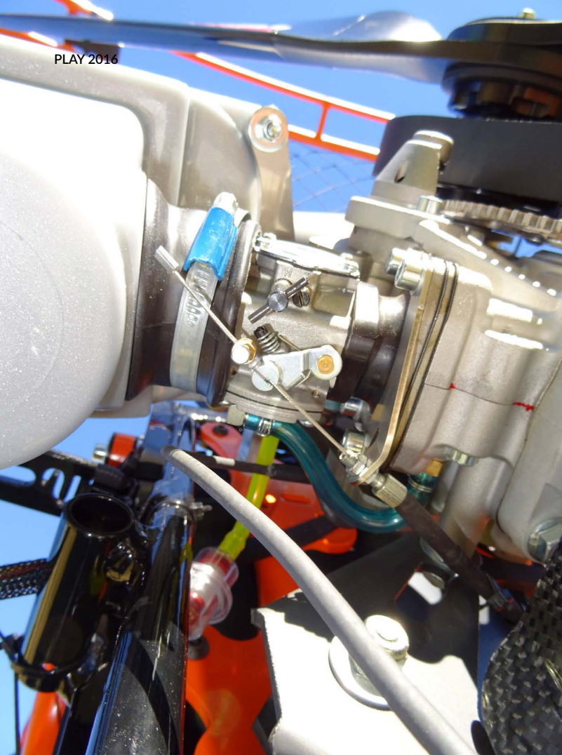
The membrane carburettor is, as always, difficult to adjust, but is requested (wrongly?!) by many clients. However that's another story...
