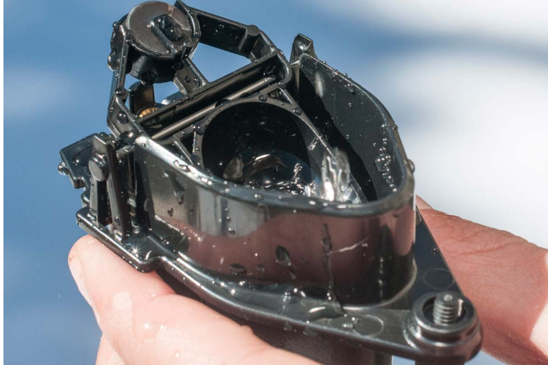
The system for the rain gauge. As soon as a precise quantity drips into the spoon, it tips over and activates a contact, thus allowing the station to record the exact quantity.
