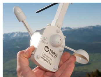
One of the first Pioupiou prototypes worked for a year with no transmission problems at an altitude of 2400 metres, day and night, although the cups had to be replaced. Right: the made in France electronics never failed.
