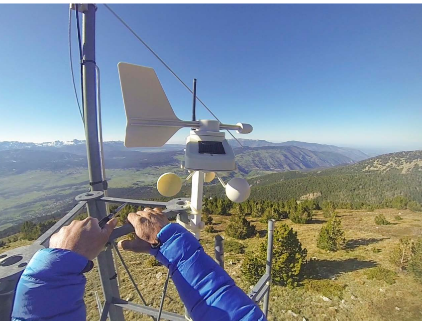
One of the first Pioupiou prototypes worked for a year with no transmission problems at an altitude of 2400 metres, day and night, although the cups had to be replaced. Right: the made in France electronics never failed.
