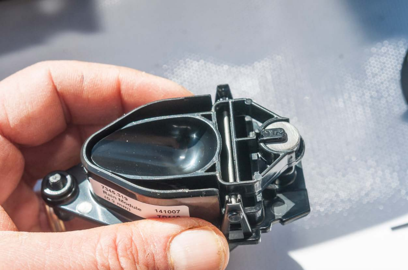
The system for the rain gauge. As soon as a precise quantity drips into the spoon, it tips over and activates a contact, thus allowing the station to record the exact quantity.
