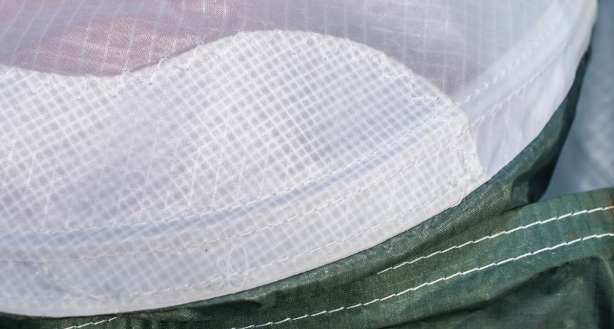
The Snake 1: sophisticated stiffening thanks to Mylar and leading edge rods, but no SharkNose.
