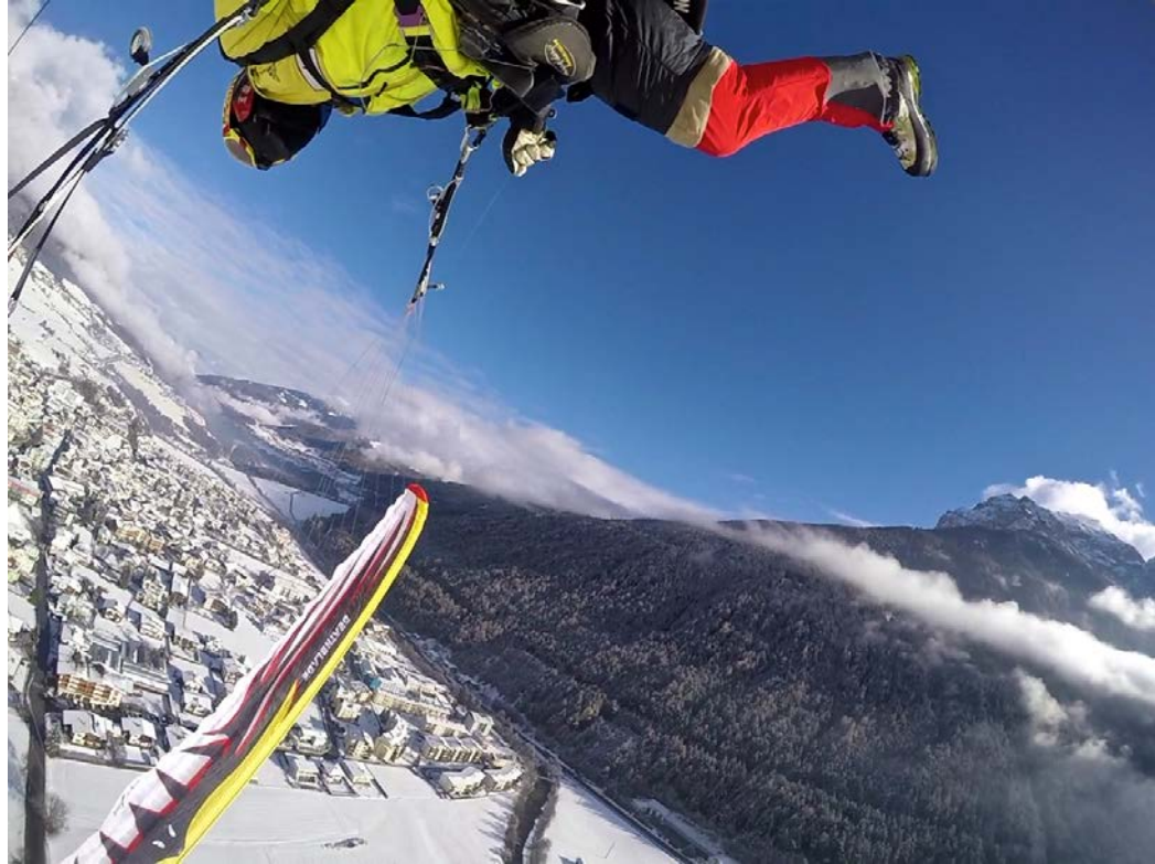
The Skyman Deathblade by Markus Gründhammer: this 2012 wing has an aspect ratio of 13.01 for a wingspan of 18.5 metres. The length of the lines is also very substantial: 18 metres.
