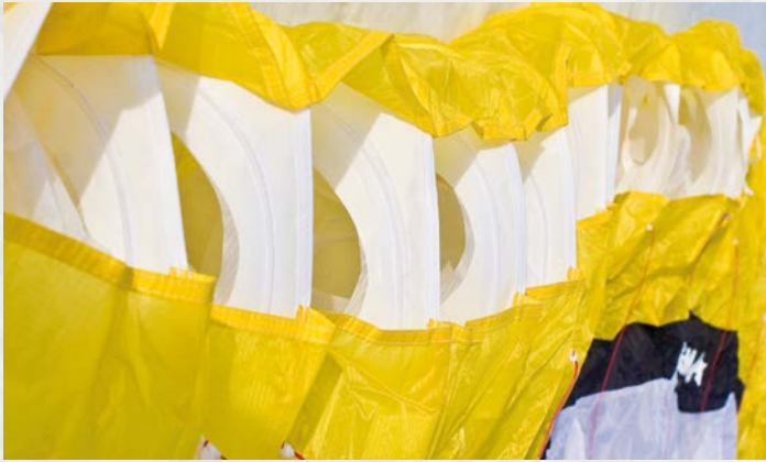
Leading edge rods or plastic wires, similar to those in a strimmer, are replacing Mylar more and more, principally for weight reasons.
