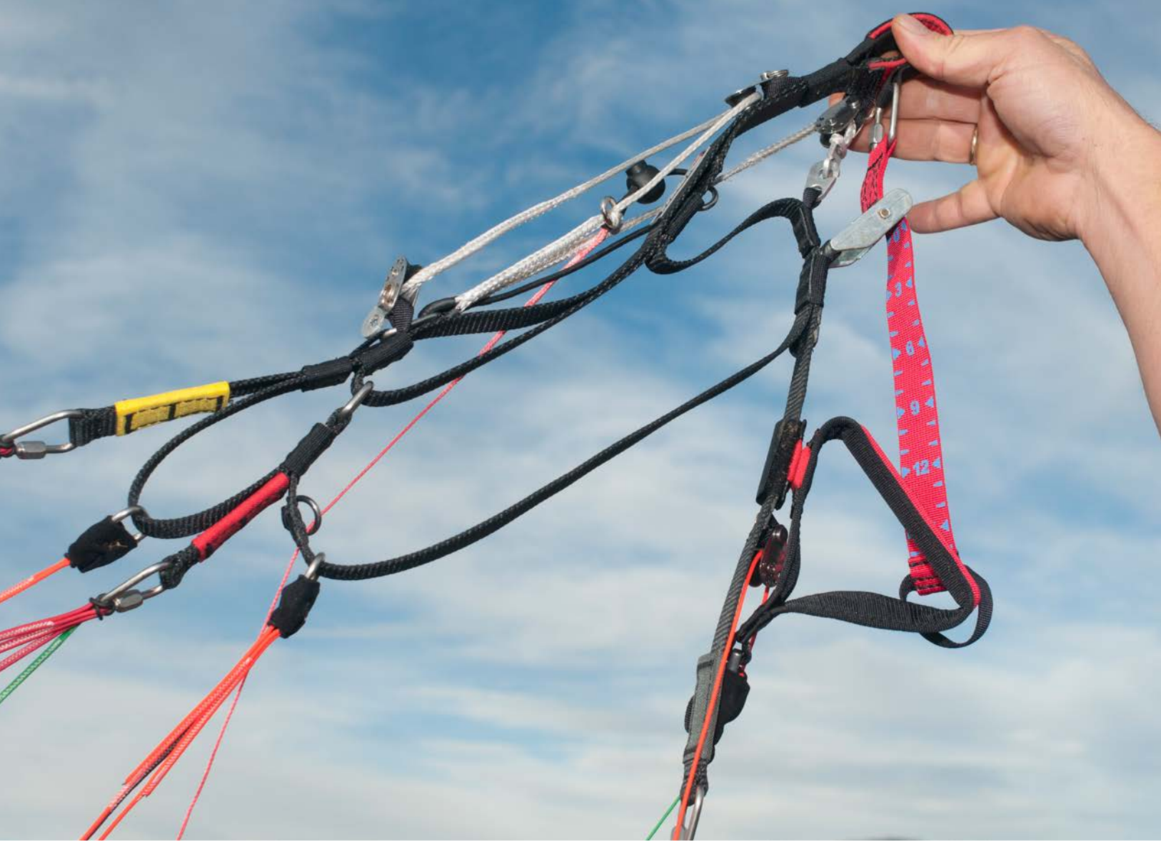
A typical riser for an efficient reflex wing.
