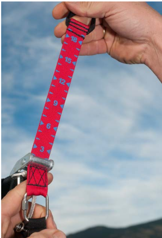
A typical riser for an efficient reflex wing.
