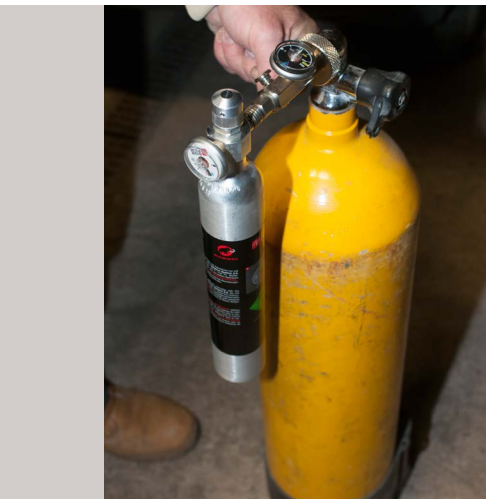
They can be recharged using a diver's bottle using its adaptor.
