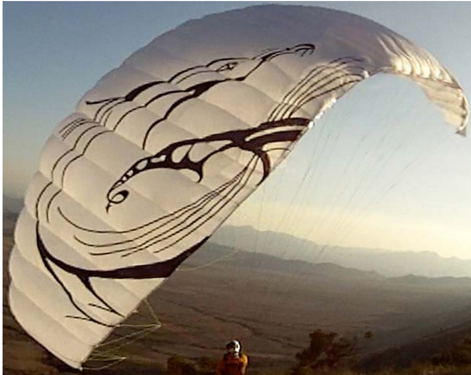
The Fastbat, a mini paraglider with a double surface.
