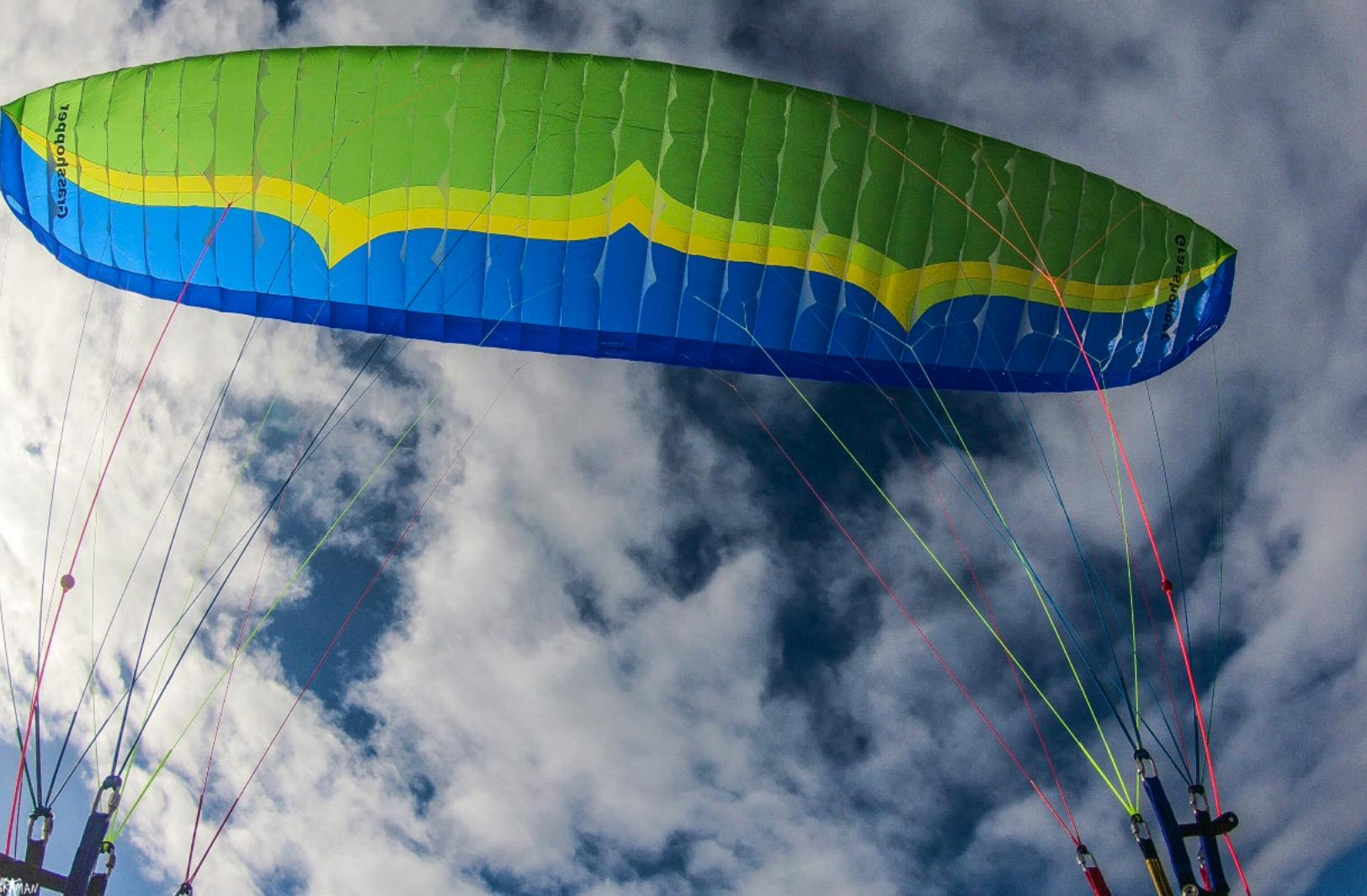
Another single skin developed by Markus Gründhammer: the Grasshopper from Independence. It's the first EN A single skin, specially designed for beginners. The balls on the brakes increase the force through the controls when approaching a stall. In addition, they transmit a force onto the Ds: an extra increase on the angle of attack and improvement of the flare when landing. At free.aero, we are testing one and should have the results soon...
