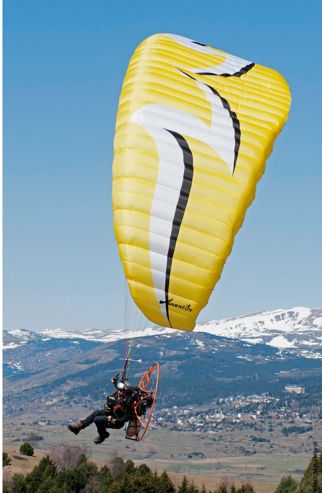
Fairly classic, but efficient: in the outer part of the wing, the brakes shorten the trailing edge to give more manoeuvrability.
