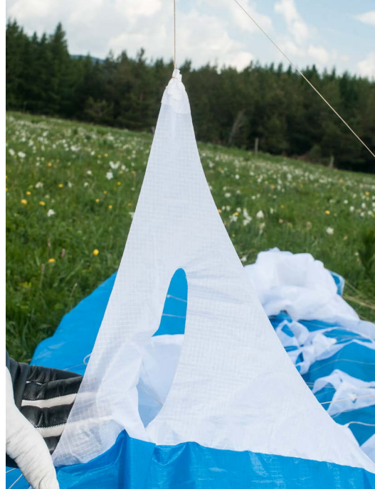
On all the single skin wings, triangular shaped pieces spread the strain of the lines over the upper surface.
