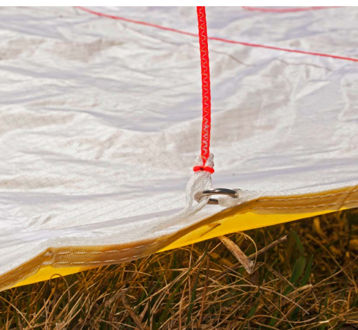
Fairly classic, but efficient: in the outer part of the wing, the brakes shorten the trailing edge to give more manoeuvrability.
