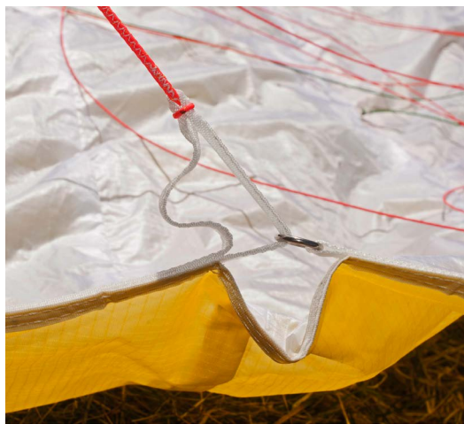
Fairly classic, but efficient: in the outer part of the wing, the brakes shorten the trailing edge to give more manoeuvrability.
