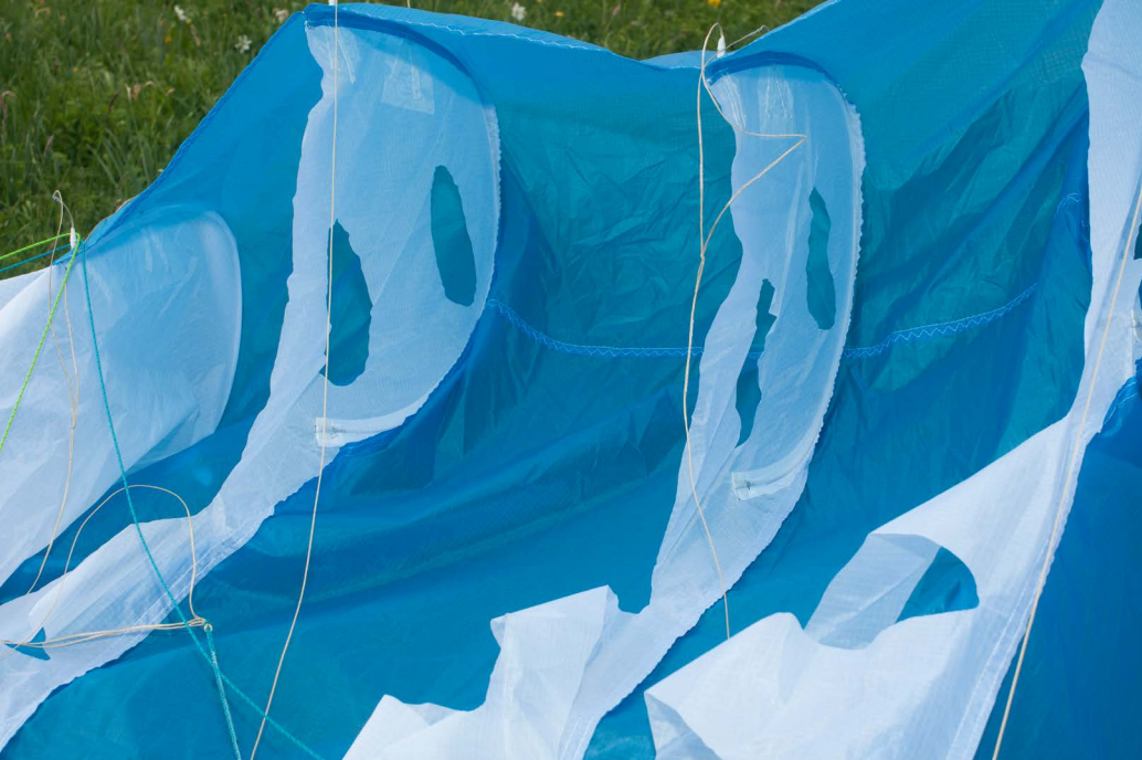
A big opening: there is no lower surface. The Nitinol leading edge rods hold the profile's nose in shape.
