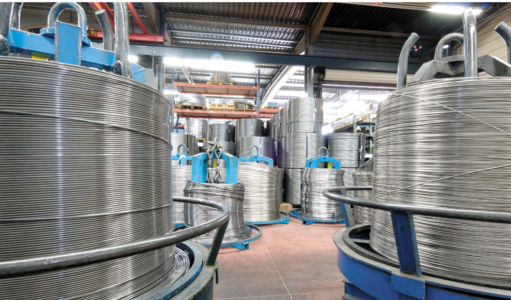
In the Peguet factory, the maillons are made from stainless-steel wire or rods...
