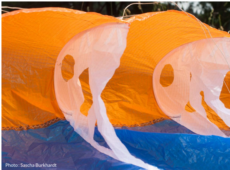
In 2013 the first Nitinol rods on production wings were launched at the Coupe Icare. Photo: Sascha Burkhardt
