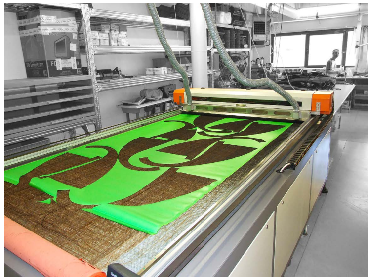
Computerised cutting at Woody Valley the harness manufacturer, using the same principle as for the paraglider profiles. (Photos: Woody Valley)
