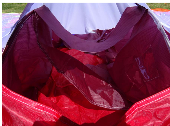
A tension band and a diagonal in an Independence Zippy.
