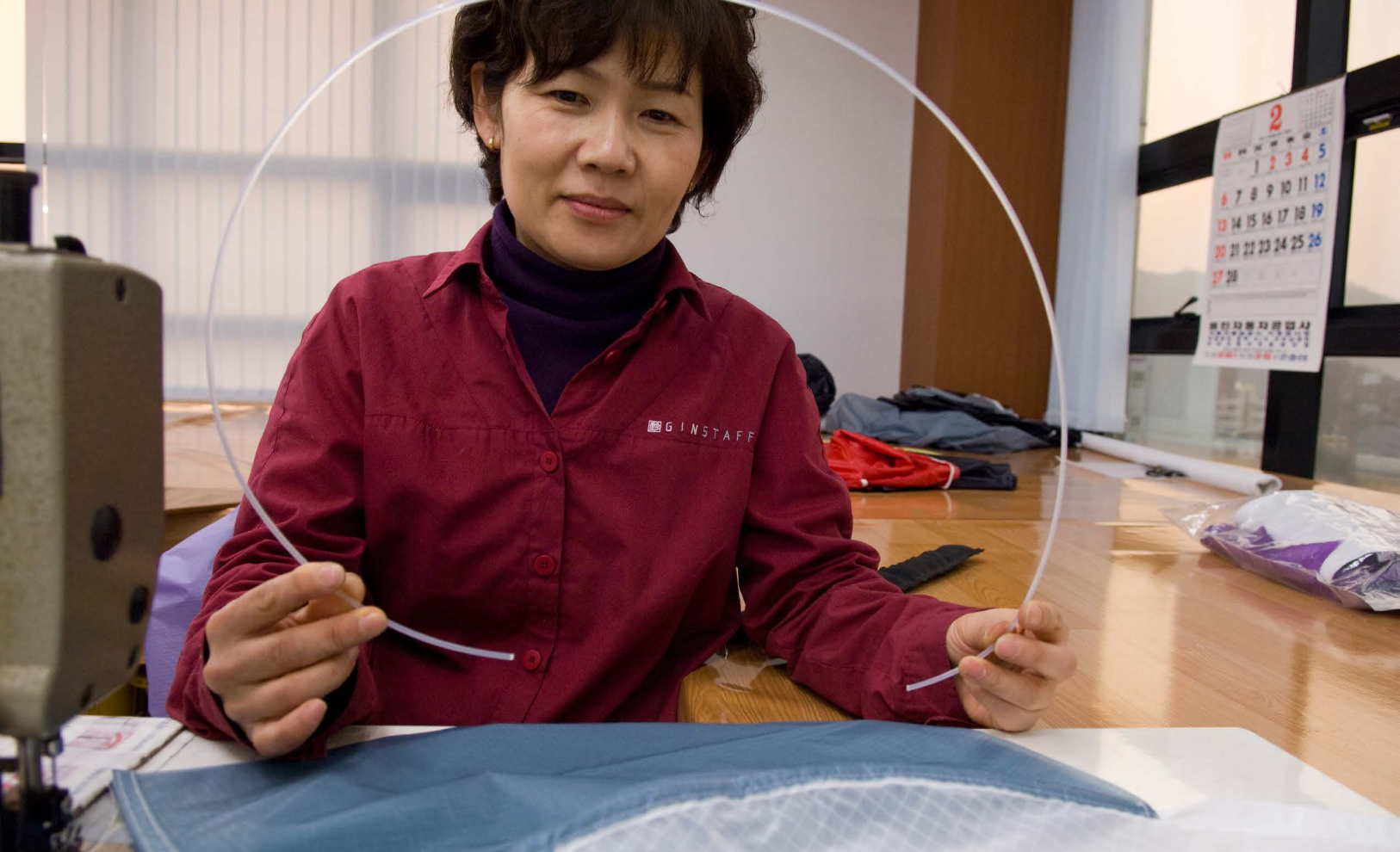
A rod about to be inserted into a wing at the Gin factory in Korea. Photo: Jérôme Maupoint/GIN Rods have become ubiquitous. Photo below.: Photo : http://albarsark.com/wordpress
