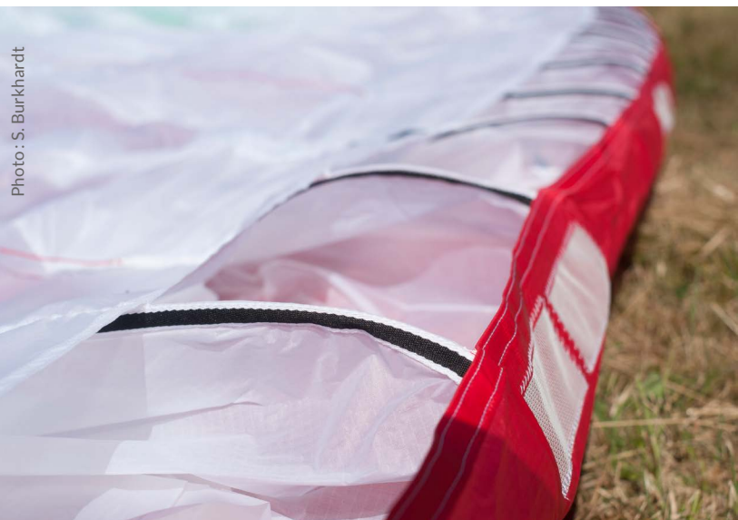
The HIT Valves by Apco are supposed to increase the internal pressure at low angles of attack
