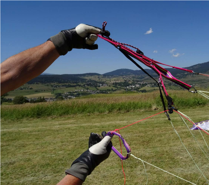
Two brake lines for one handle: one line goes to the trailing edge, the other to the stabilo...
