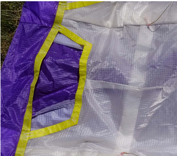
Extra bands and tension folds: a prehistoric wing, but also a precursor. The fold under the opening could be considered as 3D-Shaping twenty years ahead of its time!
