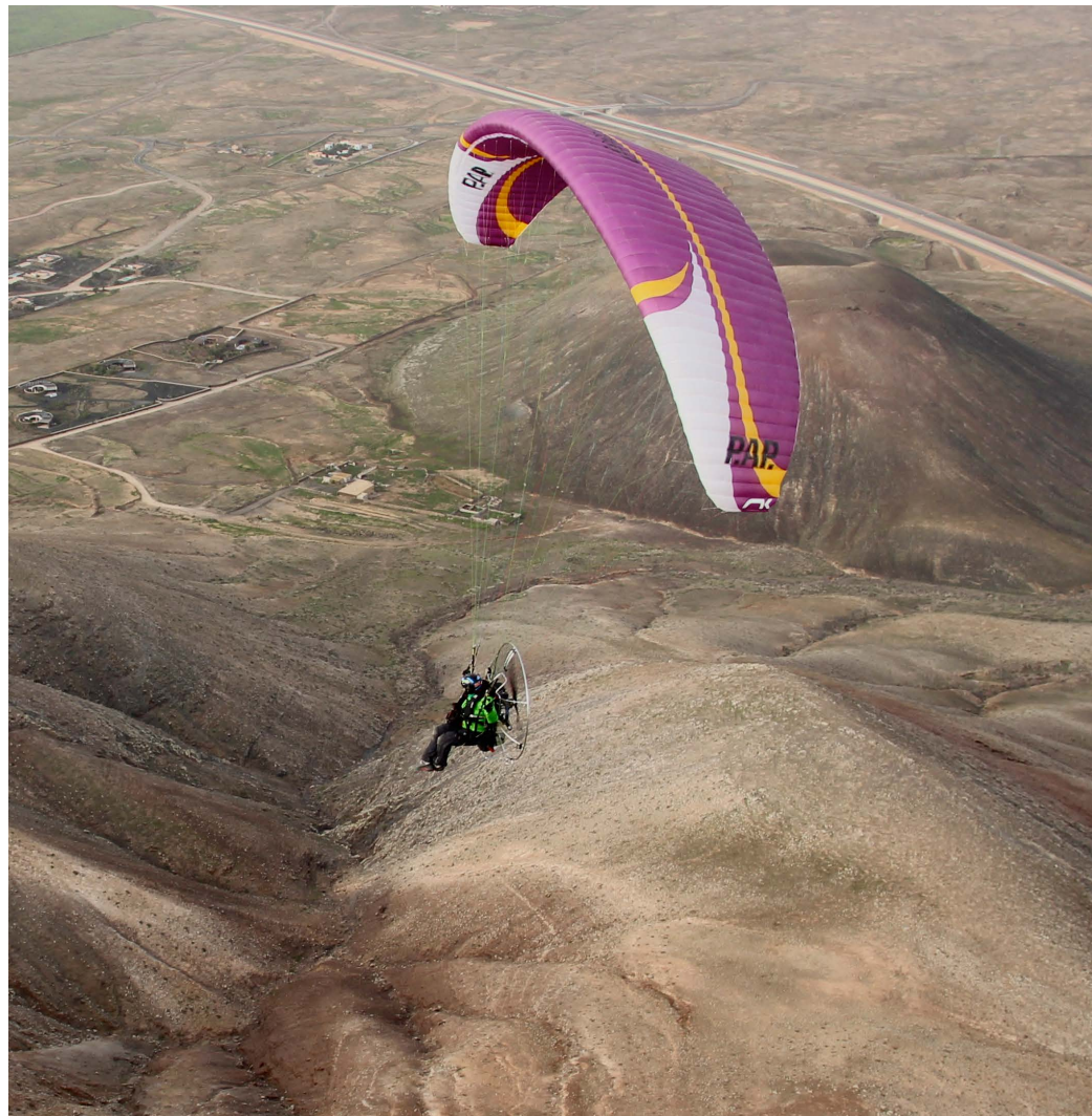
The Kougaur 2 was one of the first wings to cross a reflex profile with a SharkNose.
