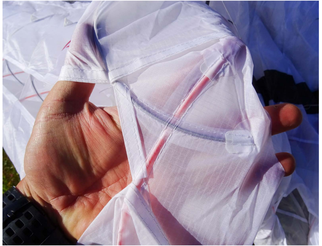
A nice SharkNose on the GIN Sprint 3 which we are currently testing. The rods crossing one another is necessary: The two rods need to have a certain amount of curvature to provide sufficient force.
