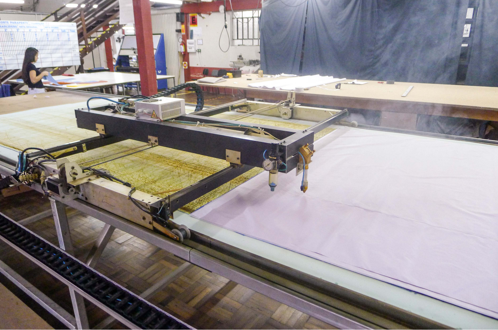
Scenes from the SOL factory in Bresil (paragliders, harnesses and accessories). Templates are used to cut the fabric for the harnesses.
