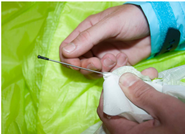
In 2013 the first Nitinol rods on production wings were launched at the Coupe Icare. Photo: Sascha Burkhardt
