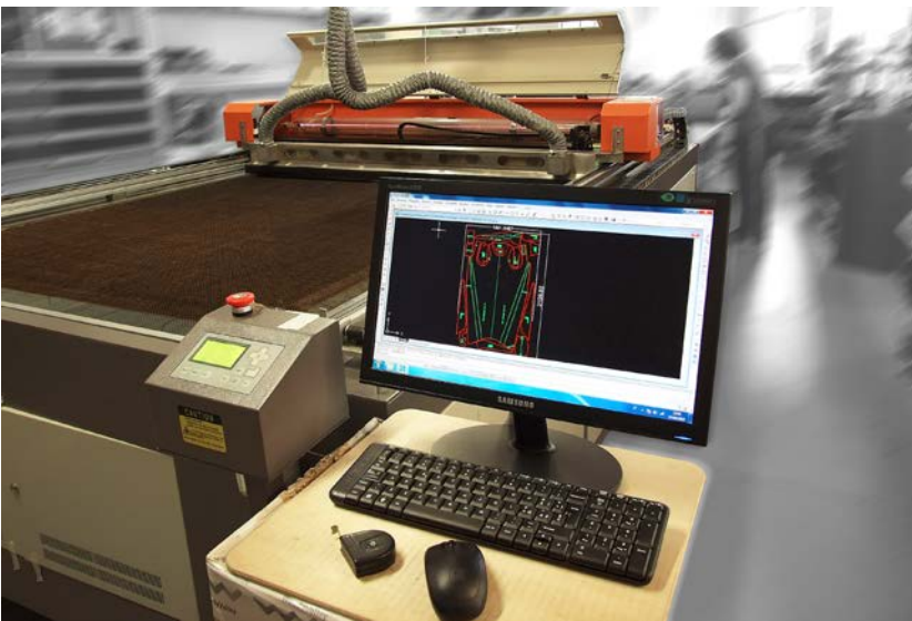
Computerised cutting at Woody Valley the harness manufacturer, using the same principle as for the paraglider profiles. (Photos: Woody Valley)
