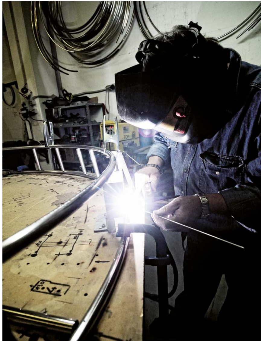
Welding the cage on a buggy. Photo : Wolfgang Ehn/ www.wolfgang-ehn.de/
