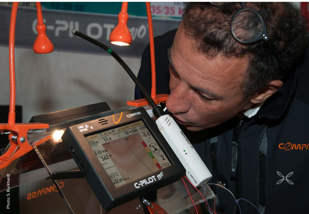
Luca Basso blowing into the instrument. The speed sensor takes into account humidity to make the TAS more precise.
