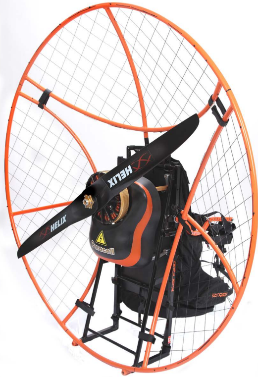
Kangook have done tests with this set up by Paracell, the Spanish assembly company. The anticipated battery life with a 72 Ah battery: more than an hour. The price still hasn't been decided.
