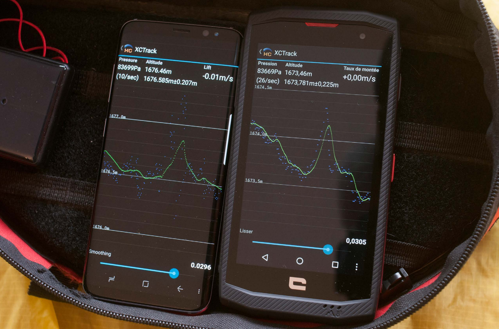
The two 'Flagships' from their respective brands: the Samsung Galaxy S8 on the left and the Crosscall Trekker X3 on the right. The Crosscall, a dedicated instrument for outdoor use, has a more precise sensor and a better sample rate of 26 Hz instead of 10 Hz. With a barometric utilisation, the difference, as far as response time is concerned, is perceptible in flight where the Crosscall reacts a bit quicker when climbing. Also visible in this photo: the points correspond to vertical movements of about 60 cm.
