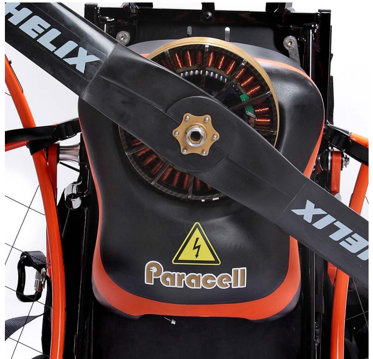
Kangook have done tests with this set up by Paracell, the Spanish assembly company. The anticipated battery life with a 72 Ah battery: more than an hour. The price still hasn't been decided.
