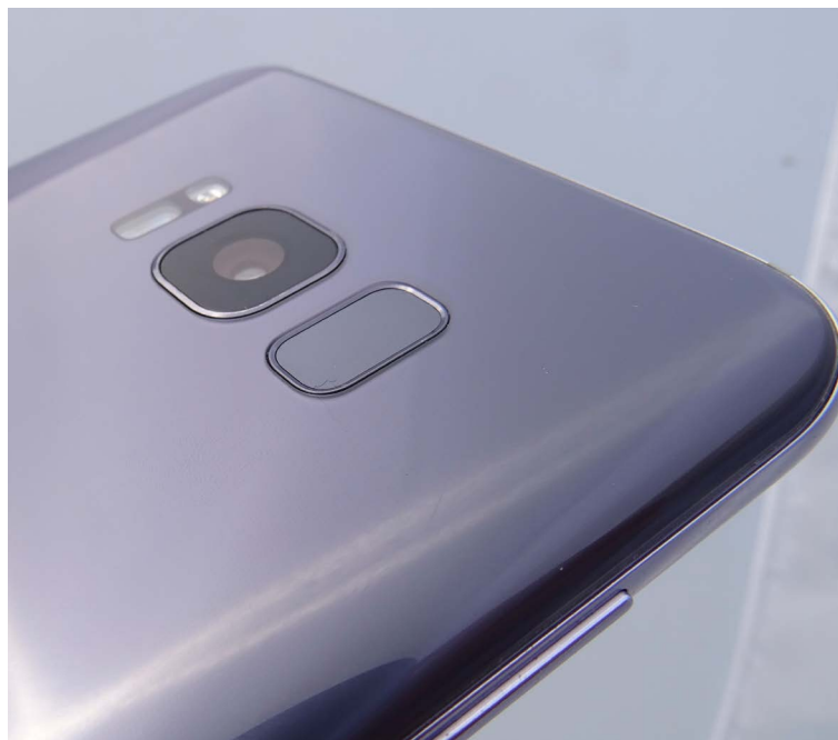
Next to the camera lens there is a digital fingerprint sensor. Practical for every day use, but not for in the air.
