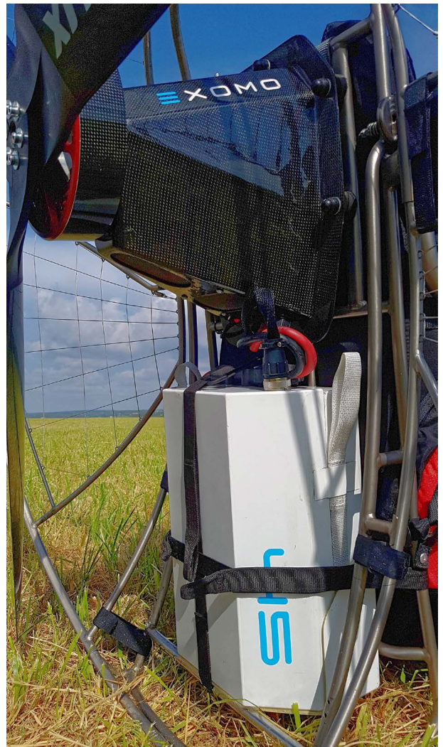
The two connections which link the battery to the motor: one for 'data' (black woven cable) the other for power (thick red and black electric cables).
