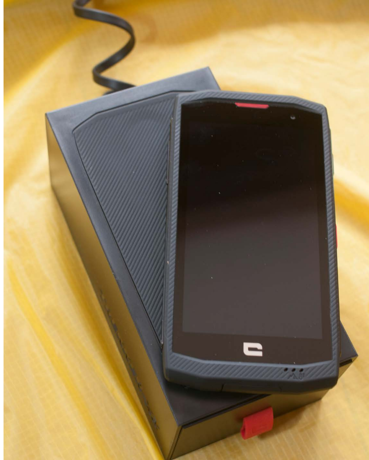
It isn't necessary to open the USB socket cover to charge the telephone: its box can be used as a cordless induction charger. It's just a bit longer.
