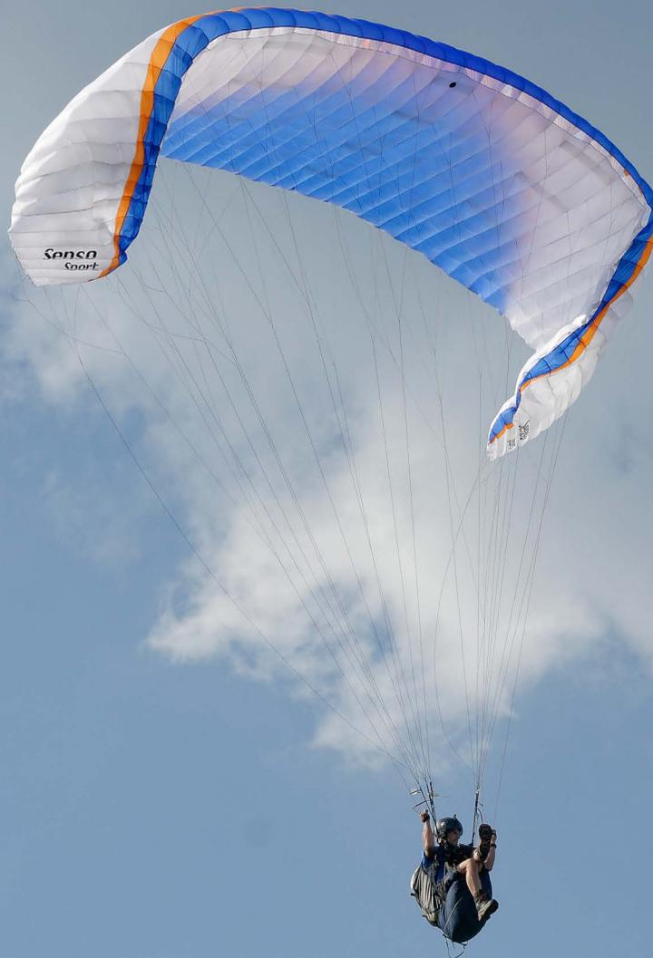
Big ears are easy to put in, the wing can be piloted pretty well by weight shift and it reopens immediately.
