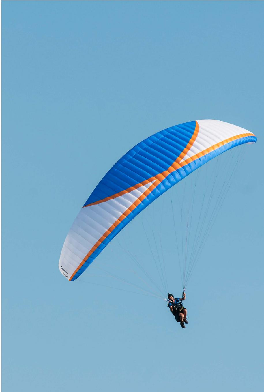
Both the Senso and the Sport are very responsive whether in mountains or with a paramotor. You can feel it is an intermediate wing which performs well. Its aspect ratio of 5.3 however puts it in the middle of the intermediate category but, as we found out, the manufacturer perhaps wasn't wrong to class it as a wing for 'school leavers'.
